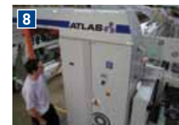
8 Drive Control Panels The electrical control panels are air-conditioned and fully integrated in to the unwind section which reduces the space required for installation and reduces the overall machine 'footprint'.
