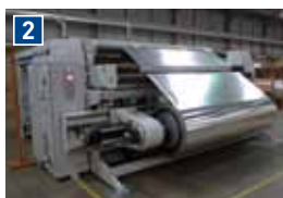
2 Shaftless Unwind A shaftless floor pick-up unwind incorporates either one or two regenerative motors for optimum unwind tension control with edge guide and optional oscillation.
